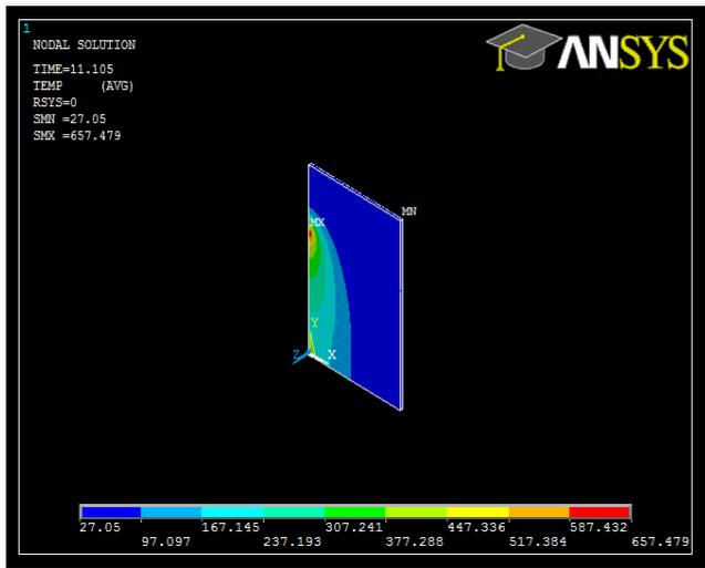
Figure 1.5 Temperature variation at 19V, 95A and 25cm/min
