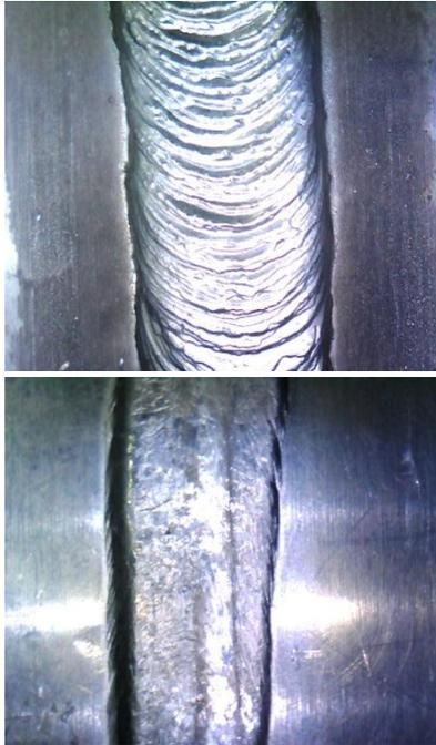
Figure 1.4 Effect of voltage and current on weld bead at (21V and 105A)
