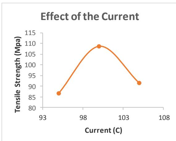
**Figure 1.2 effect of current on tensile strength**
