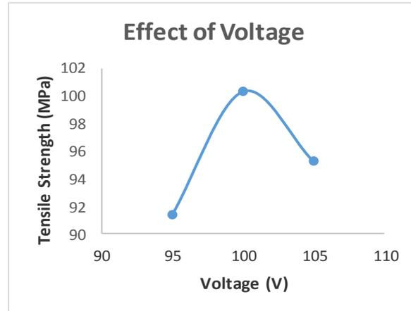
**Figure 1.3 Effect of Voltage on tensile strength**
